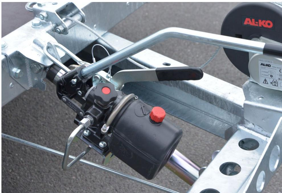
**○ Hydraulic tilt-bed** reduces loading angles and can assist in ease of operation.
