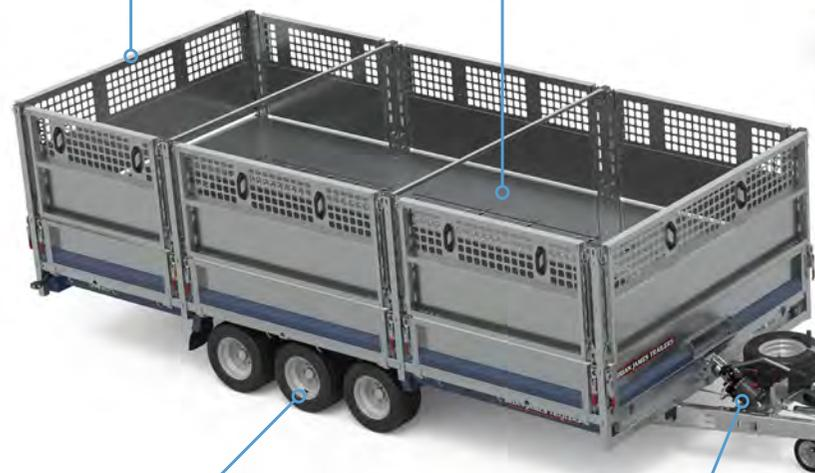
● **Heavy duty** running gear manufactured by AL-KO and featuring sealed wheel bearings ensures minimum maintenance.
