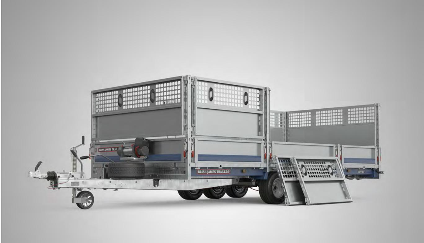
○ **Long mesh ramp with high panelled side extensions**
