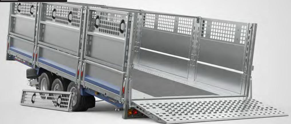
**○ Combination, tilt-bed and high grip, full width tail ramp**
